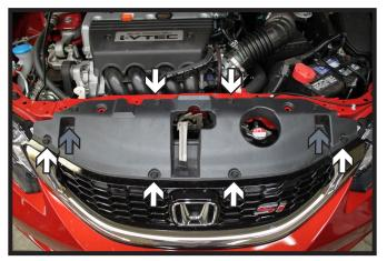
From the top edge of the fascia, remove the eight (8) push pins (white). Then using a 30 Torx, remove the two (2) screws (gray).
