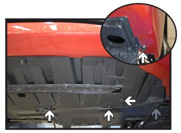
3. Using a 10MM socket, remove the screw from the underside edge of the fascia (gray). Then remove the four (4) push pins (white). Do this on both sides of the vehicle. Pull the corners of the fascia outward and forward to release from the clips. Remove the fascia from the vehicle and set aside.
