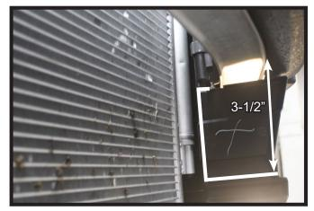
4. Measure down from the bottom of the bumper 3-1/2", mark and trim off the top of the shrouding. Do this on both sides of the vehicle.
