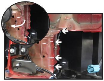
11. Using a reciprocating saw, make four (4) relief cuts thru the webbing back to the frame rail approximately as shown. Then bend the webbing forward flat against the frame face (inset). Do this on both sides of the vehicle.
