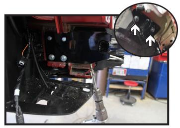
15. Using a 13/32" drill bit, drill the bottom holes thru the frame. Install 3/8"-16 x 1-1/2" bolts with 3/8" lock washers into the holes with 3/8"-16 nut plates in the frame. Do this on both sides of the vehicle. Fully tighten all hardware.
