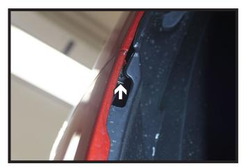
2. Using a Phillips screwdriver, remove the screw from the wheel well where the fascia meets the fender. Do this on both sides of the vehicle.
