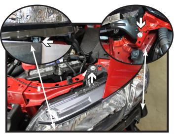
Using a 10MM socket, remove the three (3) screws from the driver side headlight only. There is a screw on the topside, the side (right inset) and underneath (left inset). Unhook any electrical wiring and set headlight aside.
