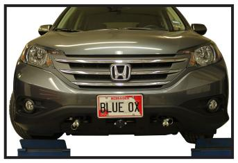
24. Hold the fascia up to the vehicle, mark and trim as needed to provide clearance for the baseplate. Reinstall the fascia making sure the baseplate convenience links and attachment tabs are situated thru the fascia before snapping the fascia back onto the vehicle.
