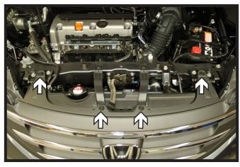
1. Remove the four (4) push pins from the top edge of the fascia.
