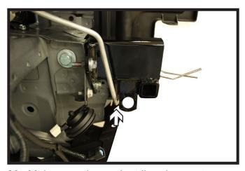
20. Make sure the coolant line does not interfere with the attachment tab. Then snap the coolant line back into the bracket.
