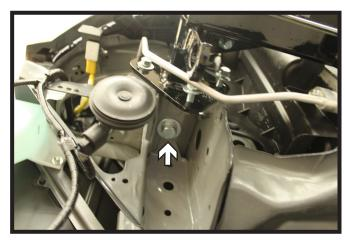
19. Insert a 1/2"-13 x 1-1/2" bolt, 1/2" lock and flat washer into the bottom hole. Use a 1/2"-13 nut plate on the inside of the frame. Do this on both sides of the vehicle. Fully tighten hardware.
