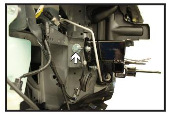
18. Insert one (1) 1/2"-13 x 1-1/2" bolt, 1/2" lock and flat washer into the side hole. Use a 1/2"-13 nut plate on the inside of the frame. Do this on both sides of the vehicle. Level the baseplate and fully tighten hardware.
