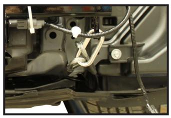
23. Attach the permanent baseplate safety cables to the provided convenience link on the baseplate. The photo shows the recommended installation of the cables to frame of vehicle. Additional options may interfere with suggested mounting; in this case, secure the cables to a solid piece of the frame as described in the instructions included with the permanent baseplate safety cables. Be sure the safety cables do not rub against any hoses or moving parts. Do this on **BOTH** sides of the vehicle.
