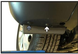
4. Remove the one (1) screw (white) and one (1) push pin (gray) that are on the under side of the fascia, in front of the tire. Do this on both sides of the vehicle
