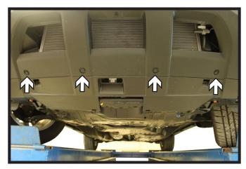
5. Remove the four (4) push pins that are located under the fascia.
