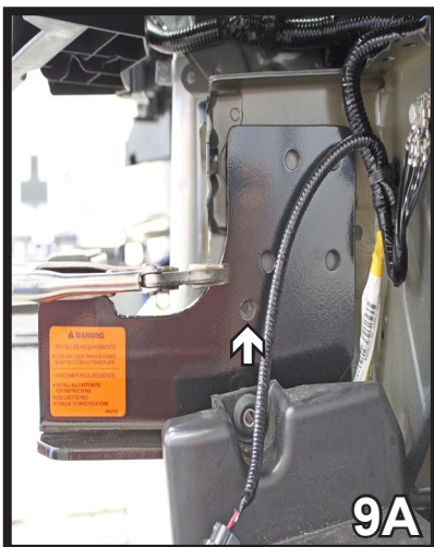
9. With the vehicle on a level surface, slide the baseplate up and in. The back of the baseplate should be flush with the frame. The existing bolt hole in the frame rail, as seen in 9A, should be lined up with your baseplate (driver's side only). Clamp with large vise grips (both sides). Be sure the baseplate is level with respect to the vehicle frame. The top of the baseplate should be approximately 7/8" down from the frame ledge as shown in 9B. Do this on both sides. Insert a 6MM-1.0 x 60MM hex bolt and 1/4" flat washer into the existing hole on driver's side frame rail as shown in 9C - Do Not Tighten .
