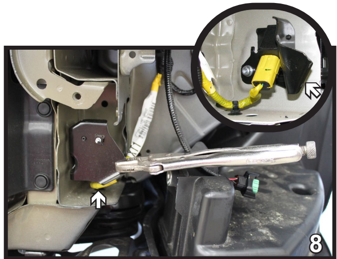
8. Clamp the air bag sensor bracket with the vice grip and bend it back, flush with frame rail. Do this on both sides.
