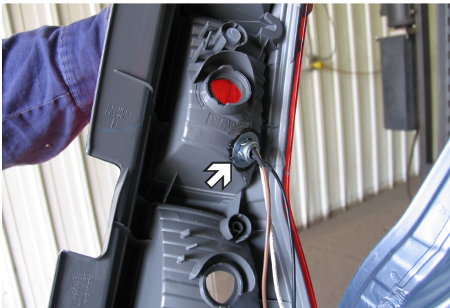
Possible location for the BX8869 Bulb and Socket Wiring Kit.
