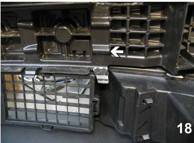
18. Using a hack saw blade, trim off tab located on the back side of the fascia. Do this to both sides of the vehicle.
