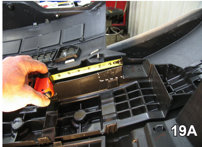
19. Using a hack saw blade, trim away plastic areas located on the back side of the fascia, just above the fascia opening as indicated in photos 19A, 19B and 19C. Do this to both sides of the fascia.
