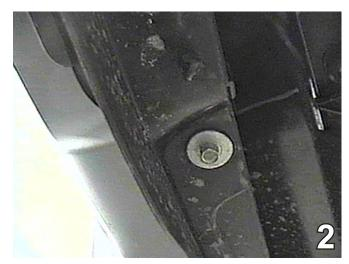
Using at 10MM socket remove two metric bolts with 10MM socket and push pins on the bottom side of fascia. There is a (the 2005 models have two) 10MM bolt to remove inside the wheel well. Do this to both sides of the vehicle. Set the metric bolts aside to be reinstalled later.
