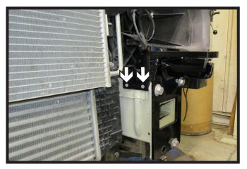
13. Using a 3/8" drill bit and the baseplate as a template, drill two (2) holes on each side of the baseplate. Do this on both sides of the vehicle.
