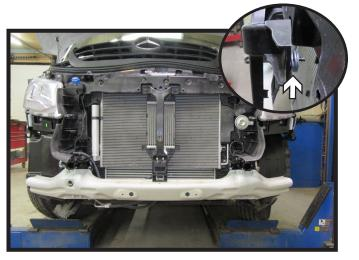
18. Reinstall the ACC Bracket by snapping bottom to the bumper and reinstalling existing bolts into the top two (2) holes with three (3) 1/4" washers on each bolt (inset). Reconnect electrical to ACC sensor.
