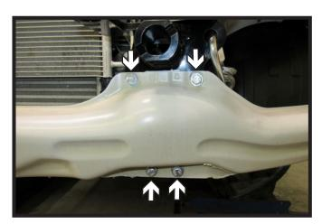
17. Slide bumper back into place and install four (4) 8MM bolts with lock washer and flat washer. Do this on both sides of the vehicle.
