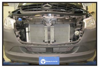
5. Unsnap and remove grille from fascia. Set grille aside to be reinstalled later.
