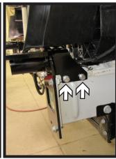
14. Install four (4) 3/8" bolts with hardware into the side holes of the baseplate. Do this on both side of the vehicle.
