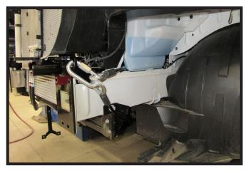
15. Attach the permanent baseplate safety cables to the provided convenience link on the baseplate. The photo above shows the recommended installation of the cables to frame of vehicle. Additional options may interfere with suggested mounting; in this case, secure the cables to a solid piece of the frame as described in the General Information sheet. Be sure the safety cables do not rub against any hoses or moving parts. Do this on **BOTH** sides of the vehicle.
