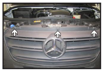
1. Using a T25 Torx, remove the three (3) bolts from the top of the fascia.
