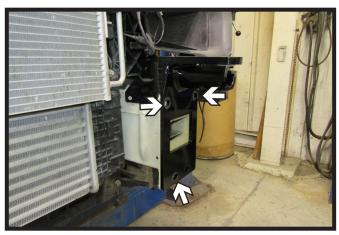
12. Line the inner edge of the baseplate with the inner frame edge. Start the front three (3) 8MM bolts. Tighten but do not apply Loctite Red at this time.
