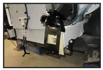
11. Tip baseplate upward and slide onto the frame of the baseplate.
