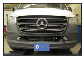
19. Hold the fascia as close to its original position, mark and trim the fascia around the convenience links and attachment tabs. Reinstall the fascia and grille.
