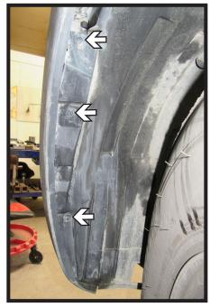
2. Remove the three (3) push pins from along the edge of the wheel well. Do this on both sides of the vehicle.
