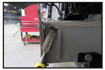
10. Use a chisel to remove the caulk from the top of the vehicle frame to allow for a better baseplate fit.
