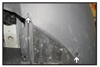
4. Remove the two (2) push pins on the underside of the fascia in front of the tire. Do this on both sides of the vehicle.
