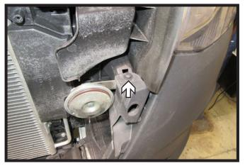
6. Using a T30 Torx, remove the one (1) bolt next to the horn. Do this on both sides of the vehicle.
