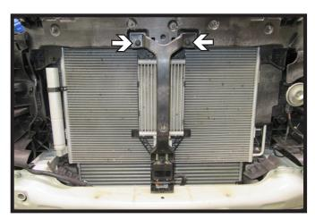
7. Using a T15 Torx, remove the two (2) bolts from the top of the Adaptive Cruise Control (ACC) bracket. Unsnap the bottom of the bracket from the bumper. Unplug electrical, remove bracket and set aside to be reinstalled later.
