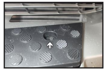
8. Using a T45 Torx, remove the two (2) screws from the step area on top of the fascia. There is one (1) on each side.
