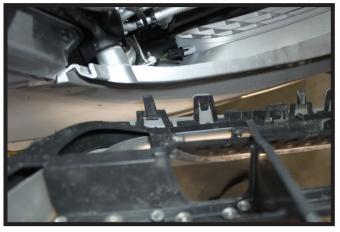
2. Pull the grille back and release the tabs at the bottom. Set the grille aside.
