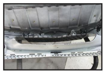
15. On the back side of the fascia, trim off the inner grille are at the joint all the way around.
