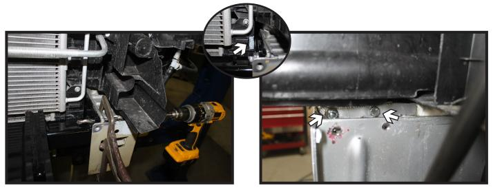
12. Clamp the baseplate to the frame of the vehicle. Using a 3/8" drill bit, drill thru the frame lips into the top baseplate holes. Install the 1/2" hardware into the top holes and fully tighten. Do this on both sides of the vehicle. Note: the plastic shielding behind may need to be trimmed for easier nut access (inset).
