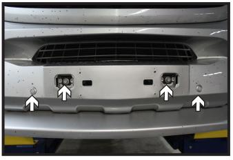
6. Using a 14MM socket, remove the four (4) screws from the front of the fascia.
