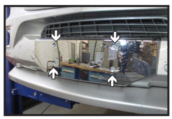
5. Using a T20 Torx, remove the four (4) screws from the front cover.
