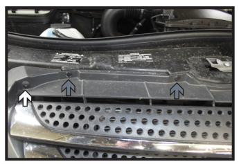
Using a T25 Torx, remove the outer screw from the top edge of the grille (white). Then remove the push pins (gray). Do this on both sides of the vehicle.
