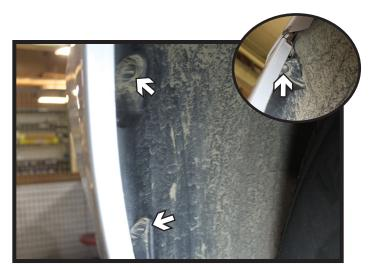
3. Remove the three (3) push pins in the wheel well. Do this on both sides of the vehicle.
