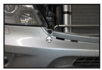
7. Using a T25 Torx, remove the two (2) screws from the front of the fascia. There is one (1) on each side.
