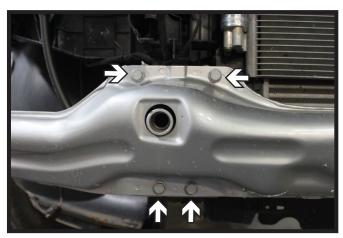
9. Using a 13MM socket, remove the eight(8) bolts from the bumper. There are four(4) on each side.
