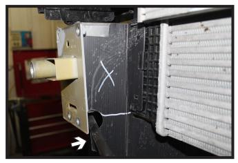
10. Remove the plastic shielding in the inner frame. Do this on both sides of the vehicle.
