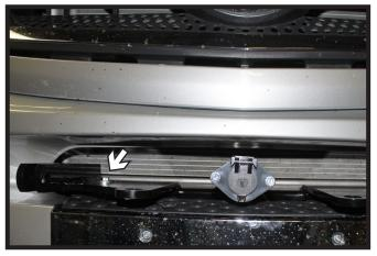
16. Reinstall the bumper and shields if taken off. Reinstall the fascia with the 3/4" spacers in the step area bolt recess areas (left). After the fascia is on the vehicle, install the 8MM hardware thru the baseplate into the step area bolt areas and fully tighten.
