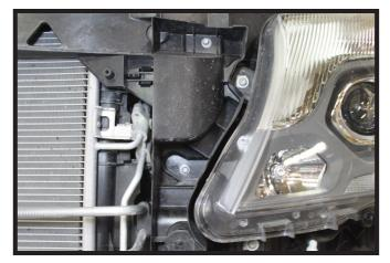
11. **Optional:** Using 13MM & 3/16" 12pt sockets, remove screws from the plastic shields on the passenger and driver sides for easier bolt installation.
