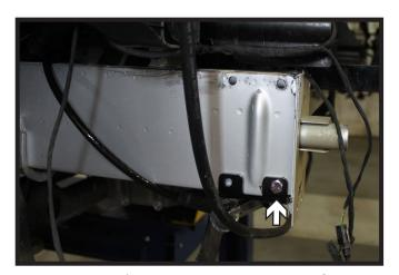
13. Using a 3/8" drill bit, drill the lower front baseplate hole thru the frame. Install the 1/2" hardware into the hole and fully tighten. Do this on both sides of the vehicle.
