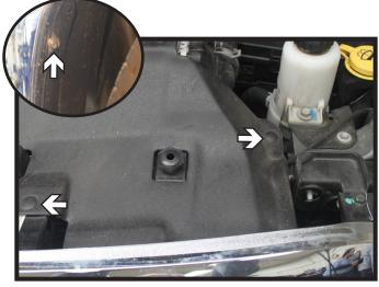
1. **2010-13 Models:** Remove the two (2) pins from the radiator cover. Do this on both sides of the vehicle. Set the cover aside.
