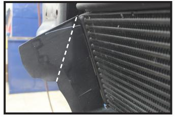
5. **2013 Models:** Trim the lower radiator shroud as shown for D-Link clearance on the baseplate. Do this on both sides of the vehicle.
