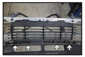
8. **2013 Models:** Using a 10MM socket, remove the two (2) screws from the top edge of the bumper (gray). Then remove the four (4) push pins from the bottom edge (white). Remove the plastic insert. Reinstall the bumper and grille to the vehicle.
