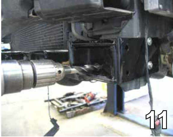
11. Using the 17/32" drill bit, drill the hole in the front of the baseplate using the baseplate as a template. Do this to both sides.
