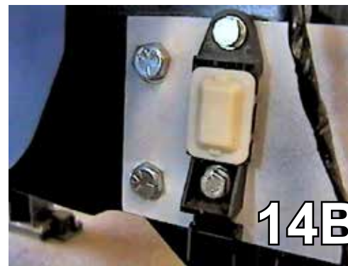
14. Using the diagonal cutters, cut off the alignment pin on the sensor and reinstall the sensor to its original position through obround
