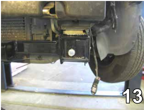
13. Insert the 1/2" nut plate into the hole on the bottom of the frame cross member to align with the drilled hole and tighten the 1/2-13 x 2 1/2" hex bolt with a lock washer. Do this on both sides.
