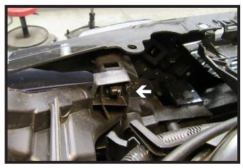
3. Using a flat screwdriver, push in the pictured clip, and pop the plastic piece out. Do this for both sides of the vehicle.
