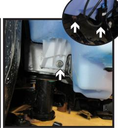
10. Remove the one (1) push pin from the top of the windshield wiper fluid reservoir. Using a 10MM socket, remove the one (1) bolt from the upper front of the reservoir, and the one (1) bolt on the back side of the reservoir. Unplug the two (2) connections from the front of the reservoir, plug the fluid lines, and remove the reservoir.
