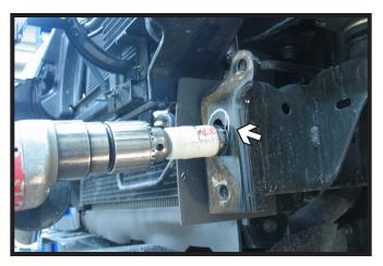
13. Using a 1-1/4" holesaw, drill a hole as shown in the driver's side frame that is connected with the existing hole for nut plate access.
