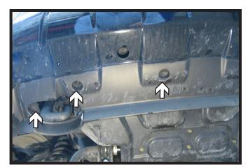
5. On the underside of the fascia, using a 10MM socket, remove the six (6) screws from the shrouding. There are three (3) on each side. Set the shroud aside.
