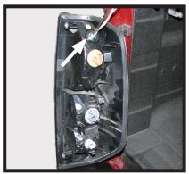
Drill a hole according to the tail light wiring kit instructions.
