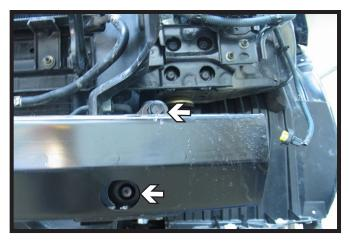
Remove the two (2) bolts from the metal bumper with a 17MM socket. Do this on both sides.
