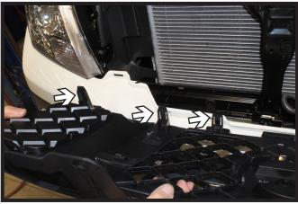
2011 & Older Models: To remove the grille, turn the two (2) square pins (inset).
