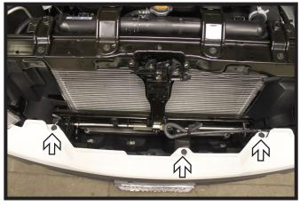
3. Remove three (3) push pins from the top of the fascia.
