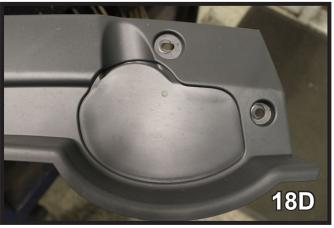
19. **Older models**: Trim the lower fascia piece where the tow hooks come through, on the driver's side cut the lip and the whole circle out like on the passenger side (18A). Continue to trim an additional 1 1/2" straight down and next to the opening (18B.
