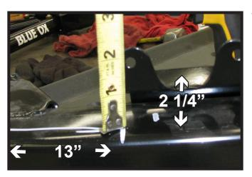
17. Set the metal bumper on a bench, clamp the electrical bracket to the back of the driver's side with the vise grip. The bracket should measure 13" from the driver's end of the metal bumper and 2 1/4" from the top edge of the bumper to the top hole location. Attach the bracket with the two (2) #10-16 self drilling screws using the 5/16" nut driver. Reinstall the metal bumper with the existing bolts. Reinstall the fascia.
