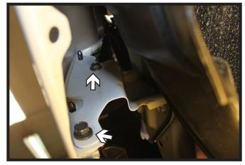
4. In the wheel well, using a Phillips screwdriver, remove the lower and upper screws. Do this to both sides of the vehicle.
