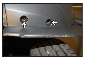
7. **Older Models:** On the back side of the rubber cover in front of the tire, remove the two (2) screws using a Phillips screwdriver. Do this on both sides. (Left)
