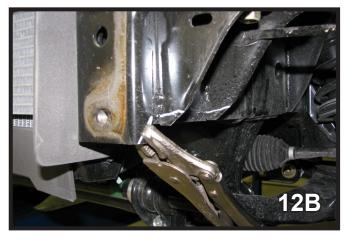
12. Using the vise grip bend the frame support, approximately 1/2" up from the bottom, back and fourth until it snaps off on both the front and back supports. Do this on both sides. (14A)
