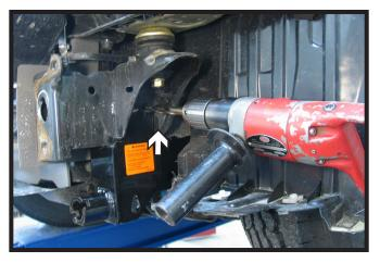
14. Using the baseplate as a template, drill a hole into the side of the frame rail with the 17/32" drill bit. Do this on both sides.
