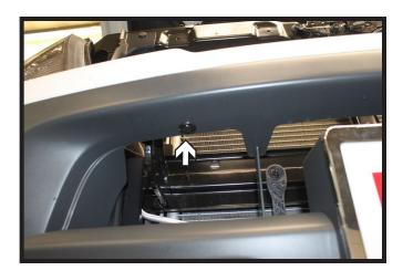
8. On the top side of the lower grille opening remove the three (3) push pins.
