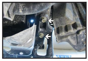
Remove the two (2) bolts from the tow hook on the passenger's side only using a 17MM socket. The tow hook will NOT be reinstalled.
