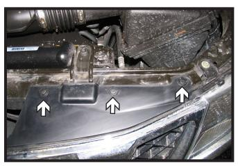
1. Remove three (3) push pins from the top of the grille. Do this on both sides.
