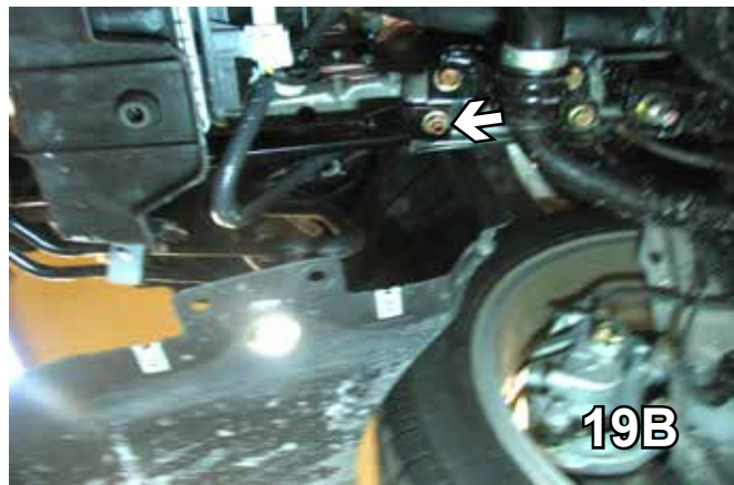
19. On the sway bar, passenger side, remove the front outside hex nut with a 14 MM socket. Install lower bracket following diagram on page 2. Use 1/2"-13 x 1 1/2" hex bolts with flat and lock washers and hex nuts, tighten with Loctite Red.
