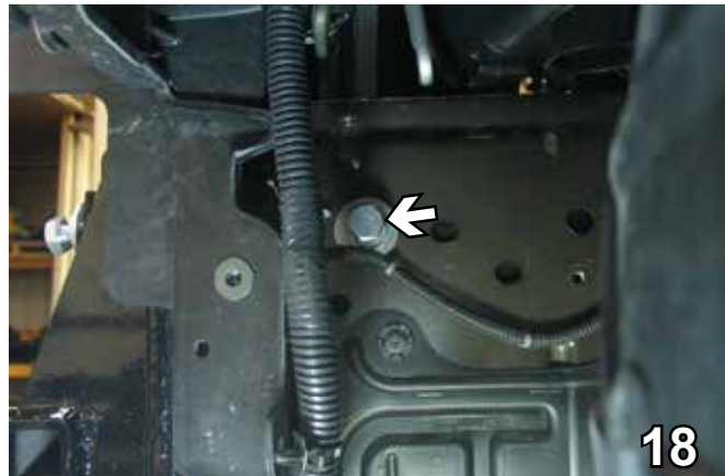
18. Align the upper bracket with existing hole in frame, then start 1/2"-13 x 1 1/2" Hex bolt with lock and flat washers. Tighten front bolt first and then the back bolt with Loctite Red. Do this to both sides.
