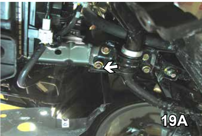
19. On the sway bar, passenger side, remove the front outside hex nut with a 14 MM socket. Install lower bracket following diagram on page 2. Use 1/2"-13 x 1 1/2" hex bolts with flat and lock washers and hex nuts, tighten with Loctite Red.
