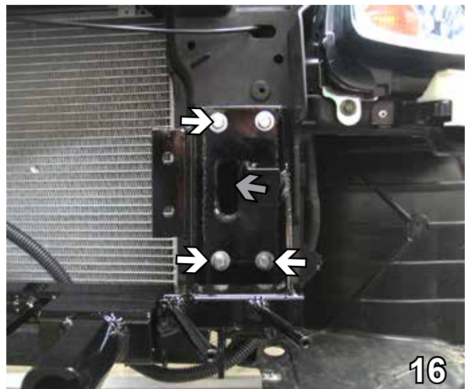
16. Insert the additional 8MM hex bolts, use Loctite Red and tighten according to specs. Do to both sides.
