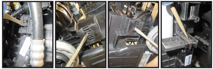
13. Using a flat screw driver, remove the four (4) clips attaching the bottom plastic shroud piece. Remove plastic piece, it will not be reinstalled.
