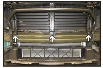
Using a 10MM socket, remove the three
