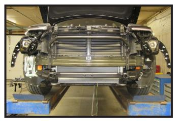
24. Reinstall windshield washer fluid reservoir, reconnecting all lines.
