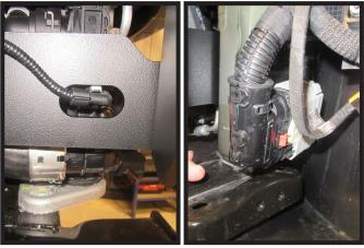
22. Reconnect electrical on passenger side and reattach electrical loom to frame on the driver side of the vehicle.
