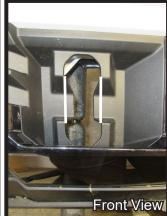
21. Using a reciprocating saw, trim the tow hook opening as shown to allow room for the baseplate. Do this on both sides of the vehicle.
