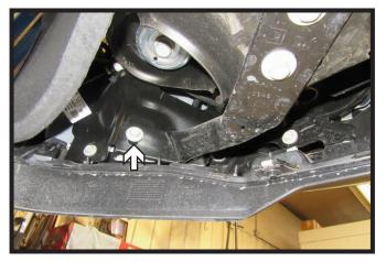
10. Using a 15MM socket, remove the one(1) bolt from the corner on the underside of the fascia. Do this on both sides of the vehicle.
