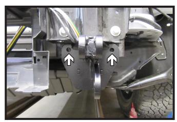
17. Using a 1/2" drill bit, drill out the front two (2) holes on the baseplate. Do this on both sides of the vehicle.
