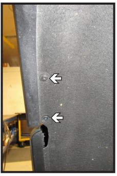
4. Using a T15 Torx, remove the two (2) bolts from along the edge of the wheel well. Do this on both sides of the vehicle.
