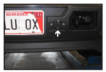
20. **Optional Silverado/Sierra Models:**Prior to fully reinstalling the fascia. Drill a hole thru the bumper at the desired location to accommodate the plug and bolts. Using 1/4" x 1-1/2" bolts with 1/4" washers, install the plug thru the bumper. On the backside of the bumper, install the electrical bracket and 1/4" locknuts to secure the plug to the bumper.
