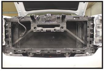
8. **All Sierra 1500 Models:** Using a 10MM socket, remove the four (4) screws from the bottom edge of the grille. There are two (2) on each side and set the grill aside (left).
