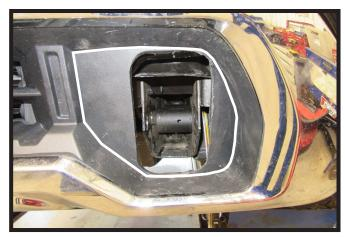
4. Using a reciprocating saw, trim the tow hook shield as indicated to allow room for the baseplate. Do this on both sides of the vehicle.
