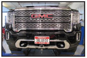
Attach electrical bracket and optional breakaway bracket to fascia in desired location
