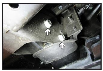
Using an 18MM socket & wrench, remove the two (2) bolts from the tow hook. Remove tow hook, it will not be reinstalled. Do this on both sides of the vehicle.
