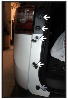
Unpop the covers for the five (5) bolts on the back panel of the vehicle. Then using a 7MM socket, remove the four (4) top bolts (white) and a T20 Torx to remove the one (1) bottom bolt (gray). Do this on both sides of the vehicle.
