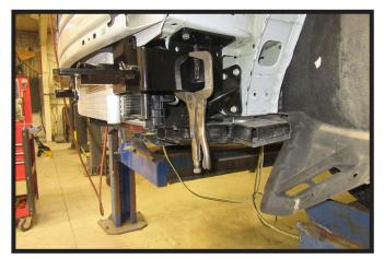
10. Slide baseplate into place. Use large vise grips to hold in place. Do this on both sides of the vehicle.
