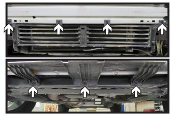
Using a 7MM socket, remove seven (7) bolts, four (4) on top and three (3) on bottom, from the shutters. Unplug and set aside to be reinstalled later.
