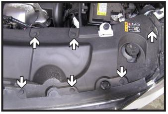
1. Remove the twelve (12) push pins from the fascia cover on the top of the vehicle. There are six (6) push pins on each side of the vehicle. Remove fascia cover and set aside to be reinstalled later.
