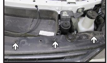
2. Using a 7MM socket, remove the six (6) bolts, three (3) on each side, from the top of the fascia.
