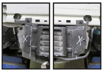
7. Unhook the wire loom on the driver side of the vehicle. Trim the shutter housing as indicated on both sides of the vehicle.
