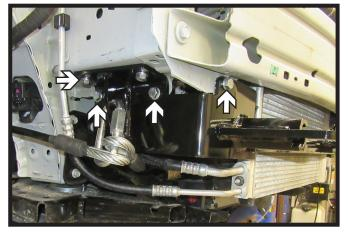
Using a 3/8" drill bit, drill the remaining four (4) holes. Install 3/8" hardware. Do this on both sides of the vehicle.
