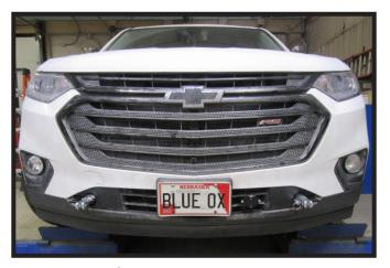
18. Hold the fascia as close to its original position, mark and trim the fascia around the convenience links and attachment tabs. Use a 2-1/2" hole saw to create the holes for the attachment tabs. Reinstall the fascia, fascia cover, and reconnect all electrical connections.
