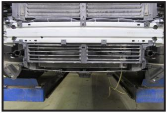
15. Hold the shutters in place and trim sides around the attachment tab housing as needed.
