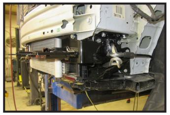
14. Attach the permanent baseplate safety cables to the provided convenience link on the baseplate. The photo above shows the recommended installation of the cables to frame of vehicle. Additional options may interfere with suggested mounting; in this case, secure the cables to a solid piece of the frame as described in the General Information sheet. Be sure the safety cables do not rub against any hoses or moving parts. Do this on **BOTH** sides of the vehicle.
