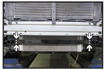
12 . Install the cross bar using four (4) 3/8" bolts, two (2) on each side, with lock washer and two (2) flat washers in between the side bracket and cross bar for each bolt as a spacer.
