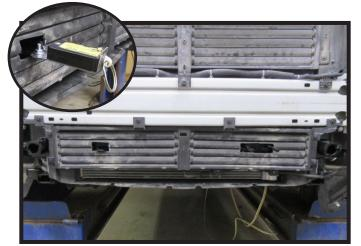
16. Notch the middle two shutters as show for electrical rids and the breakaway bracket. Reinstall the shutters on the vehicle.
