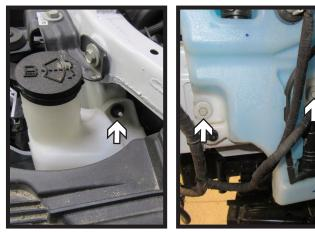
8. On the driver side of the vehicle, using a 10MM socket, remove the one (1) nut from the top of the windshield washer fluid reservoir. Disconnect all lines. Then using a 10MM socket, remove the two (2) bolts at the bottom of the reservoir.
