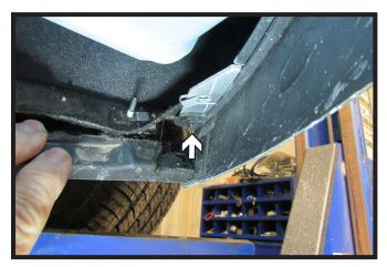
4. Pull the plastic piece down and using a 7MM socket, remove the one (1) bolt.
