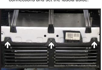
6. Using a 7MM socket, remove the three (3) bolts from the shutter housing. Let shutter hang loose.
