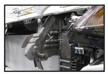
Using a utility knife remove the plastic piece as indicated. Do this on both sides of the vehicle.
