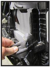
8. Using a utility knife trim the indicated areas on each side of the grill to allow room for the baseplate.
