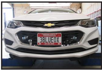
16. Hold the fascia as close to its original position, mark and trim the fascia around the convenience links and attachment tabs. Reinstall the fascia and fascia cover.
