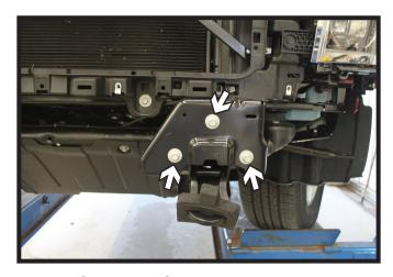
11. **All Silverado/Sierra Models:** Using a 15MM socket, remove the three (3) bolts from the cover plate. Do this on both sides of the vehicle.
