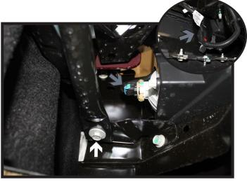
All Silverado/Sierra Models: Using a 15MM socket, remove the bolt from the bumper reinforcement bar. Do this on both sides of the vehicle. Disconnect the running lights/electrical connections (gray).
