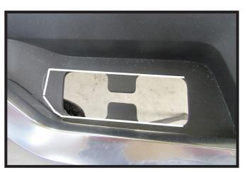
17a. All Tahoe/Suburban Models: On the inside of the fascia trim the indicated area to allow the attachment tabs and convenience links to fit through. Do this on both sides of the fascia.
