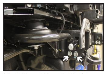
12b. **All Silverado/Sierra Models:** Using a 18MM socket/wrench, remove the two (2) bolts from the tow hook. Do this on both sides of the vehicle (left). Set the tow hooks and hardware aside they will not be reinstalled.
