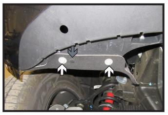
All Tahoe/Suburban Models: Using a 10MM socket, remove the six (6) screws from the underside of the fascia. There are three (3) on each side. Remove the two (2) push pins located in front of the tires (gray).
