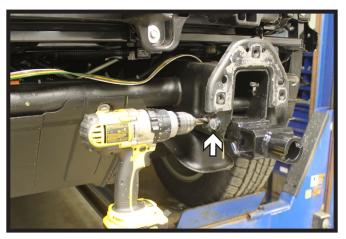
14. **All Models:** Insert the front 1/2" bolt and start the bottom 1/2" bolt with step washer, do this on both sides of the vehicle. Do not fully tighten the bolts. Note: The bottom frame hole may need to be reamed out to align with the slot.
