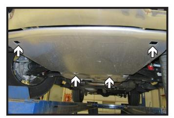
5. **All Z71 Models:** Using a 16 MM socket remove the four (4) bolts, two (2) in the front and back, attaching the belly pan.
