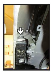
Using a T15 Torx, remove the two screws from the edge of the wheel well in front of the tire. Next, pull the cover back. Using a 7MM socket, remove the one (1) bolt from under the cover. Do this for both sides of the vehicle.
