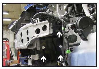
9. Using a 3/8" drill bit, drill out the remaining three (3) holes and insert the provided 3/8" hardware. Do this for both sides of the vehicle.
