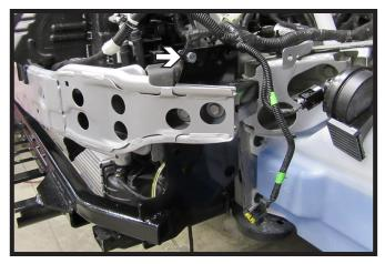
Slide the baseplate into position and ensure it is level, then slide spacer plate into position between frame and baseplate before clamping to the frame rail on both sides with large vise grips.
