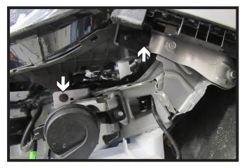
6. Using a 7MM socket, remove the four (4) bolts from the headlight. There are two (2) on top of the headlight area, and two (2) below the headlight on the side. Remove the headlight and set aside. Do this for both sides of the vehicle.
