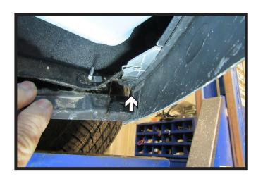
4. Pull the plastic piece down and using a 7MM socket, remove the one (1) bolt.
