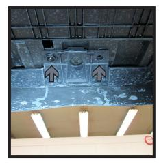
3. Using a 7MM socket, remove the six (6) bolts (white) from the underside of the vehicle. There are three (3) on each side of the car. Remove the two (2) push pin (gray) from the center of the underside.
