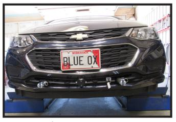
12. Hold the fascia as close to its original position, mark and trim the fascia around the convenience links and attachment tabs. Reinstall the center brace, headlights, fascia and fascia cover.
