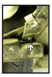
4. Using a 7MM socket, remove the two (2) bolts under the vehicle in front of the tire. Next pull the plastic piece down. Remove the one (1) bolt.
