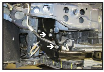
10. On the passenger side, attach the flat plate with the provided 3/8" hardware.
