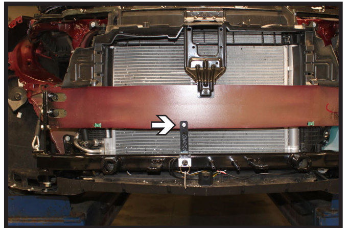
18. Optional Breakaway: In the desired location, drill a 1/4" hole thru the bumper lip. Install the bracket to the bumper with the provided 1/4" hardware. Attache the breakaway to the bracket with the 1/4" hardware provided.
