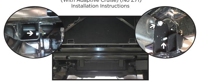
7. Align the baseplate to the existing holes in the frame. Start the two (2) existing bolts on the driver side that were removed from the ACC bracket (right). On the passenger side install a 1/2"-13 x 1-1/2" bolt with lock washer into the existing hole and a 1/2"-13 whiz nut on the inside (left). Level the baseplate and fully tighten all hardware.
