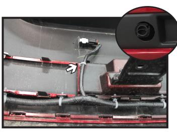
12. On the backside of the fascia, disconnect the wiring loop. Reinstall the fascia as close to its original position. Mark and trim the fascia around the attachment tabs.
