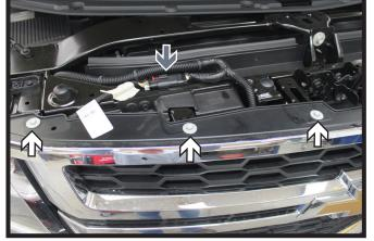
Using a 10MM socket, remove the six (6) screws from the top edge of the fascia (white). There are three (3) on each side.
