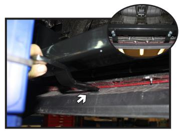
13. Reinstall the fascia as close to its original position. Hold the convenience link as close to it's installed position. Mark and trim the fascia around the convenience link. Do this on both sides of the vehicle.
