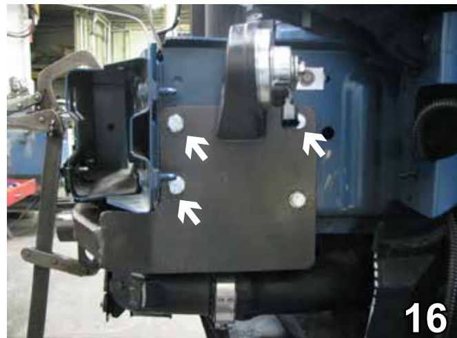
16. Insert three more 3/8-16 x 1 1/4" hex bolts with 3/8" lock washers and attach to 3/8-16 nut plates. Be sure to use Loctite. This is done on both sides of the vehicle.
