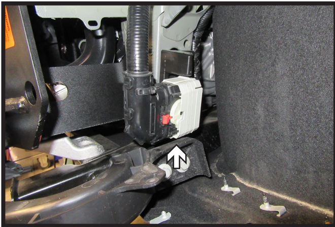
14. Unclip electrical loom from frame on driver side of the vehicle to allow for installation of support plate.
