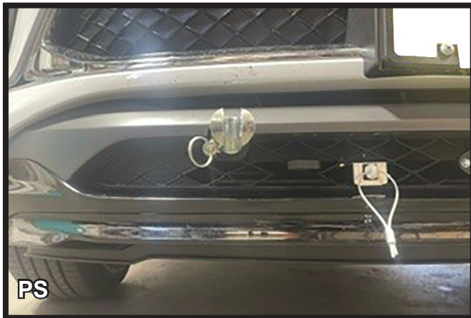
25b. Fascia Style 2: Hold the fascia as close to its original position and mark. Using a reciprocating saw trim each side of the fascia as shown to allow room for the baseplate and
