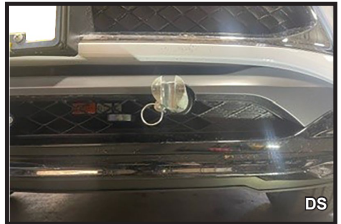
25b. Fascia Style 2: Hold the fascia as close to its original position and mark. Using a reciprocating saw trim each side of the fascia as shown to allow room for the baseplate and
