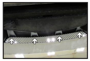
5. Remove four (4) push pins from the inside of the fascia.
