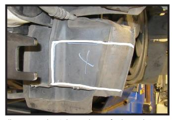
15. Using a reciprocating saw, trim the plastic shrouding approximately as shown for baseplate clearance.
