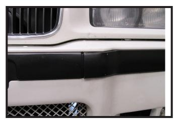
9. On the front of the car, pop the black plastic bumper off. Under the bumper, there will be three (3) push pins to be removed (removed bumper not pictured). Do this for both sides of the vehicle. Pull the corners of the fascia away from the vehicle disconnecting any electrical connections and set the fascia aside.
