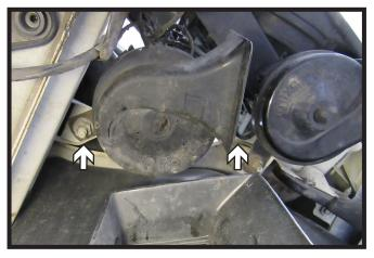
12. On the driver's side, using a 13MM socket, remove the two (2) bolts for the horns.
