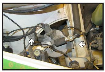
11. Using an 8MM socket, remove the two bolts from the inside on the passenger side.
