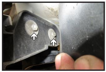
Under the wheel well, pull back the plastic cover. Using a 10MM socket, remove the two (bolts). Do this for both sides of the vehicle.
