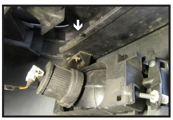
7. Using an 8MM socket, remove the screw from the top of the fascia (View from below is pictured). Do this for both sides of the vehicle.
