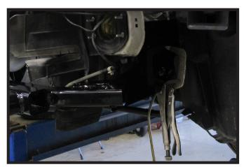
16. Slide the baseplate Into position and insure it is level and aligned with existing holes, before clamping to the frame rail on both sides with large vise grips.
