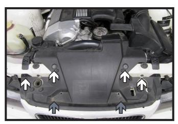
Using a T25 Torx, remove the two (2) screws from the top edge of the fascia (gray). Using a Phillips screwdriver, remove the four (4) push pins (white).
