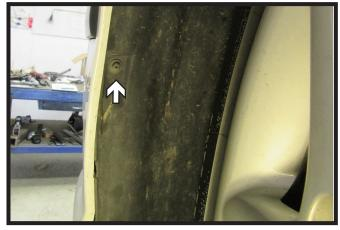
Underneath the wheel well, using a Phillips screwdriver, remove the one (1) screw. Do this for both sides of the vehicle.
