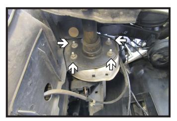
13. Using a 10MM socket, remove four (4) bolts from the bumper horn. Do this for both sides of the vehicle.
