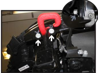
Using a 16MM socket, remove the two (2) bolts from the underside of the tow hook (white). Using a 30MM socket, remove the nut from the backside of the tow hook and remove from the vehicle (inset). Do this on both sides of the vehicle.
