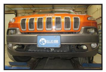
12. Hold the fascia as close to its original position, mark and trim the fascia electrical and optional breakaway. Reinstall the fascia, fascia cover and reconnect all electrical.
