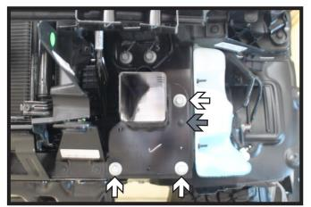
Using a 15MM socket, remove the three
