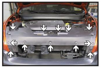
Remove the twelve (12) push pins from the top edge of the fascia cover. There are five (5) on each side and one (1) in the center. Remove fascia cover and set aside to be reinstalled later.
