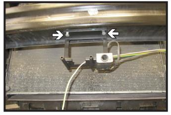
Hold electrical/breakaway mounting bracket in place and mark bumper. Using a 1/4" drill bit, drill two (2) holes for the bracket. Attach bracket to the bumper using the two (2) 1/4" bolts and hardware.
