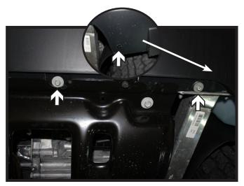
Remove the two (2) rivets from the underside corners of the fascia (inset). There is one (1) on each side. Using a 10MM socket, remove the four (4) bolts from the middle portion of the fascia. There are two (2) on each side.
