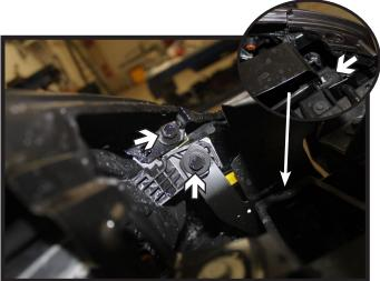
Using a 10MM socket, remove the three (3) bolts from the backside of the fascia next to the fender. There are two (2) in the corner and one (1) directly below the bracket (inset). Do this on both sides of the vehicle.
