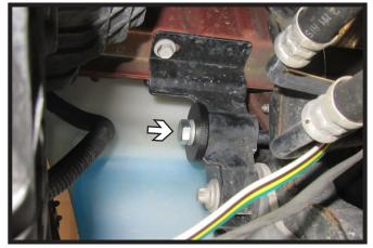
From the backside install the 1/2" x 5" bolt with lock washer and 1/4" x 2" DIA washer plate. Do this on both sides of the vehicle.
