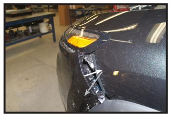
Lift the corners of the fascia up towards the fender (white) and out to release (gray). Continue along under the headlights unsnapping the fascia from the vehicle. Unplug electrical on driver side. Set the fascia aside to be reinstalled later.
