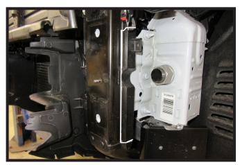
11. Using a reciprocating saw, trim the frame as indicated. Do this on both sides of the vehicle.
