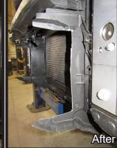
12. Using a utility knife, cut and remove the area from plastic shroud as shown. Do this on both sides of the vehicle.
