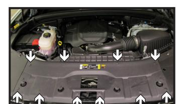
1. Remove the ten (10) push pins from the top of the fascia cover. Remove fascia cover and set aside to be reinstalled later.
