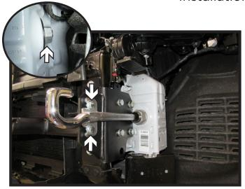
21. Reinstall tube with nut on the driver side of the vehicle. Then reinstall tow hooks on each side of the vehicle using two (2) 3/8" bolts with lock washers, flat washers, and a nylon lock nut for the top bolt and a nut plate for the bottom bolt. Reinstall existing nut on back of each tow hook (inset).
