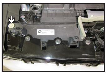
3. Using a 10MM socket, remove the one (1) bolt from the top of the fascia. Do this on both sides of the vehicle.
