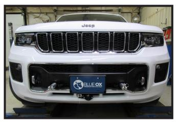
24. Hold the fascia as close to its original position, mark and trim the fascia around the convenience links and attachment tabs. Reinstall the fascia, fascia cover, belly pan and reconnect all electrical connections.
