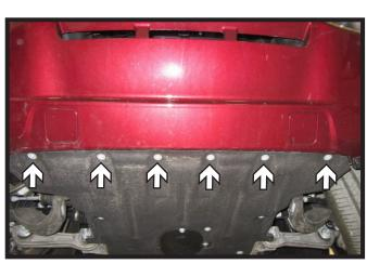
7. Using a 10MM socket, remove the six (6) bolts from the belly pan.
