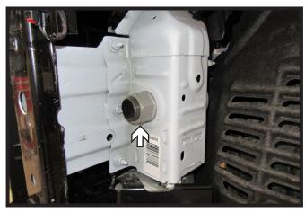
14. Using an extra large crescent wrench, remove the nut from the driver side of the vehicle. Slide tube back and out of the way to be reinstalled later.
