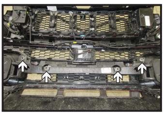
23. Remove the four (4) clips attaching the foam piece to the back of the fascia. Remove foam piece, it will not be reinstalled.
