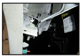
5. Pull back the wheel well liner. Using a 10MM socket, remove the one (1) bolt from the fascia joint. Do this on both sides of the vehicle.
