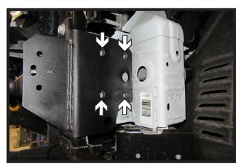
17. Using 1/2" drill bit. Drill the four (4) holes (white) on the side of the frame using the baseplate as a template. Do this on both sides of the vehicle.
