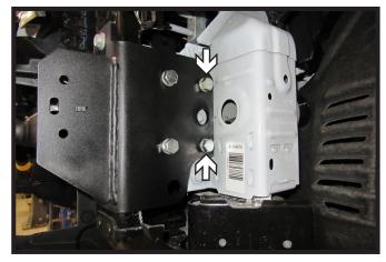
20. Install two (2) 1/2" x 1-1/2" bolts with lock washers and whiz nuts back holes. Do this on both sides of the vehicle. Tighten all bolts at this time.
