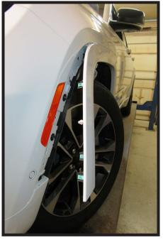
6. Unsnap the wheel well trim just past fascia joint. Hold trim away from fascia using a soft cloth. Do this on both sides of the vehicle.
