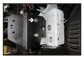
19. Insert spacer plate at top of baseplate between the frame and baseplate with the slotted end facing downward. Once spacer plate is in position insert 1/2" x 1-1/2" bolt with lock washer and whiz nut into top front hole.
