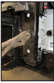
13. Using vice grip pliers, shake bolt to loosen. Then using a hammer, pound out bolt and remove. Do this on both sides of vehicle.
