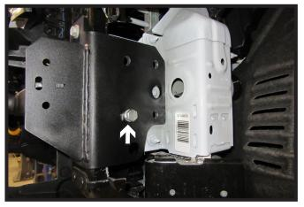
18. Start a 1/2" x 1-1/2" bolt with lock washer and whiz nut in the bottom front hole. Leave loose at this time. Do this on both sides of the vehicle.
