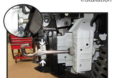
9. Using a 16MM socket, remove the two (2) bolts (white) from the tow hook. Then using a large crescent wrench, remove the nut (gray) from the back of the tow hook (inset). Remove tow hook and set aside to be reinstalled later. Do this on both sides of the vehicle.
