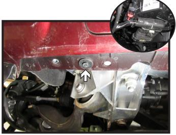
8. Let belly ban hang and remove one (1) push pin from each side of the vehicle.
