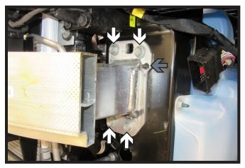
9. Using a 15MM socket, remove the four (4) bolts from the bumper. Using a 10MM socket, remove the nut (gray) from the bumper. Do this on both sides of the vehicle. Remove the bumper and set aside to be reinstalled later.
