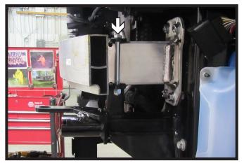
Place bracket on top of the bumper and secure to baseplate using two (2) 3/8" x 4-1/2" bolts with nylon lock nuts. Do this on both sides of the vehicle.
