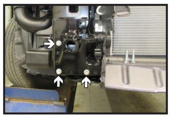
10. On one side of the vehicle, slide the baseplate into place and start the three(3) existing 10MM bolts with flat washers and lock washers. Snug baseplate against frame but do not fully tighten at this time.
