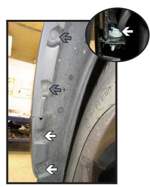
2b. **Some Vehicles:** Using an 8MM socket, remove the two (2) bolts (white) and two (2) push pins (gray) from the edge of the wheel well. Pull back the wheel well cover, using a 10MM socket, remove the bolt behind the trim (inset). Do this on both sides of the vehicle.
