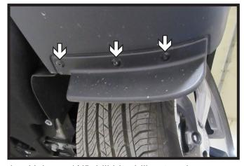
4. Using a 1/4" drill bit, drill out and remove the three (3) pop rivets underneath the vehicle in front of the tire. Do this on both sides of the vehicle.
