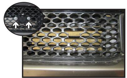
17. **Non Shutters Models:** Trim the fascia on one side of the vehicle as shown to allow room for the electrical bracket. Install bracket using two (2) 1/4" bolts with hardware (inset).
