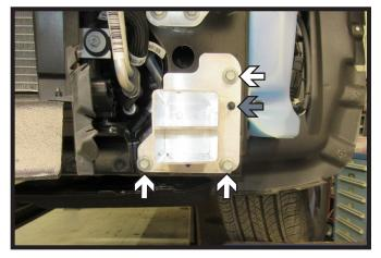
Using a 15MM socket, remove the three
