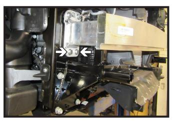
14. Install the bottom two (2) 10MM bolts with flat washers and lock washers into the bottom holes of the bumper. Do this on both sides of the vehicle.
