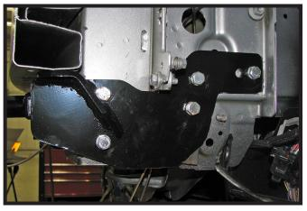
14. Continue drilling the remaining holes thru the frame and installing the appropriate hardware/spacers as needed. Do this on both sides of the vehicle. Fully tighten all hardware.
