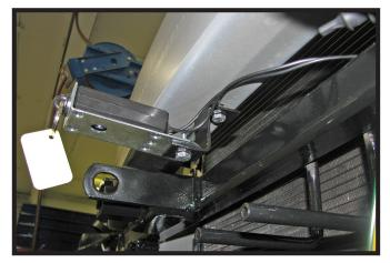
18. **Optional Breakaway:** Drill a 1/4" hole at the desired location along the bottom side of the bumper and install the bracket with the supplied 1/4" hardware.
