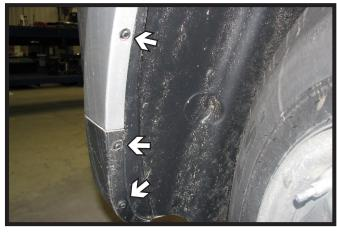
Using a 7MM socket, remove the three (3) screws from along the edge of the wheel well. Do this on both sides of the vehicle.
