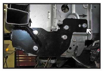
13. Position the baseplate onto the frame. Pushing it tight against the underside of the bumper and frame lip in the rear. Level and clamp firmly in place.
