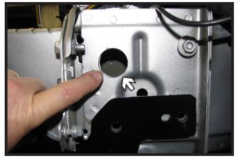
12. Using a 1-1/4" hole saw, drill an access hole in the frame as shown. Do this on both sides of the vehicle.
