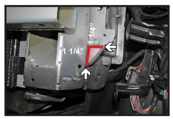
Using a reciprocating saw, notch the frame just below the bolt approximately 1-1/4" both ways. Do this on both sides of the vehicle.
