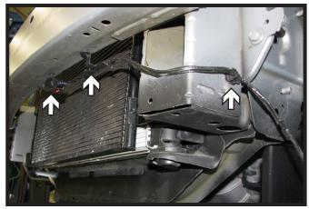
8. Disconnect the temperature sensor from the underside of the bumper/frame and set aside.
