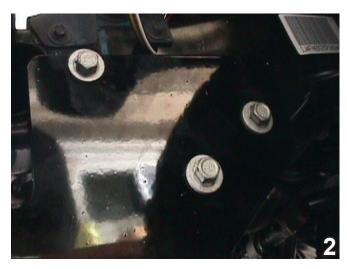
2. Hold the baseplate into place and insert the three (3) existing bolts on the driver's side through the baseplate, frame and gear box. Tighten the bolts.
