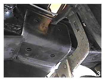
Clamp the baseplate on the passenger's side with the large vise grips. Using the baseplate as a template, drill four (4) holes with the 13/32" drill bit.
