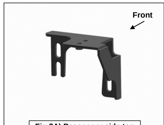
Fig 3A) Passenger side top frame bracket illustrated
