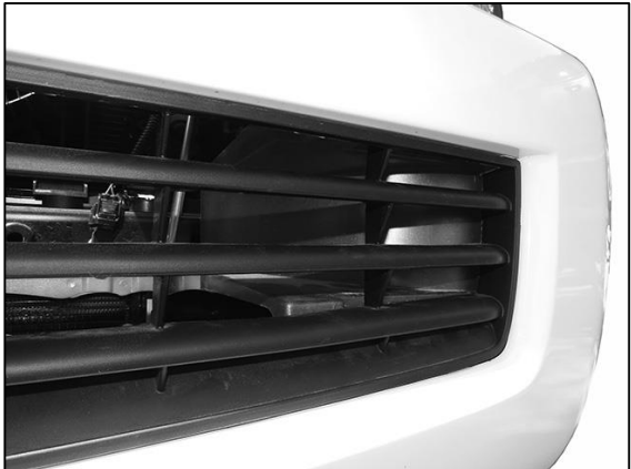
(Fig 5A) Remove or cut air deflector from behind lower grille opening in bumper
