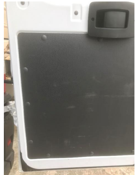
Figure 11: Remove Plastic Door Rivets
