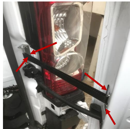
Figure 18: Completed Door Strap Installation
