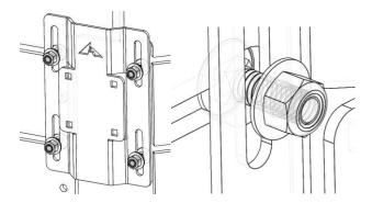
Orient the carriage bolt and slide the accessory over until the next set of carriage bolts can be installed through the relief cut on the second set of slots.
