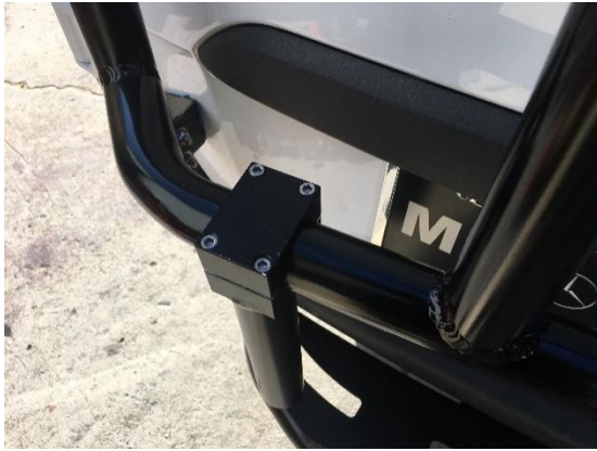
Figure 7: Bolt-On Supports Loosely Bolted to Lower Crossmember
