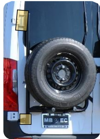
Figure 1: Protective Tape Locations on Door
