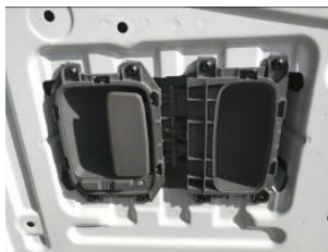
Figure 4: Inner Door Handle Removal
