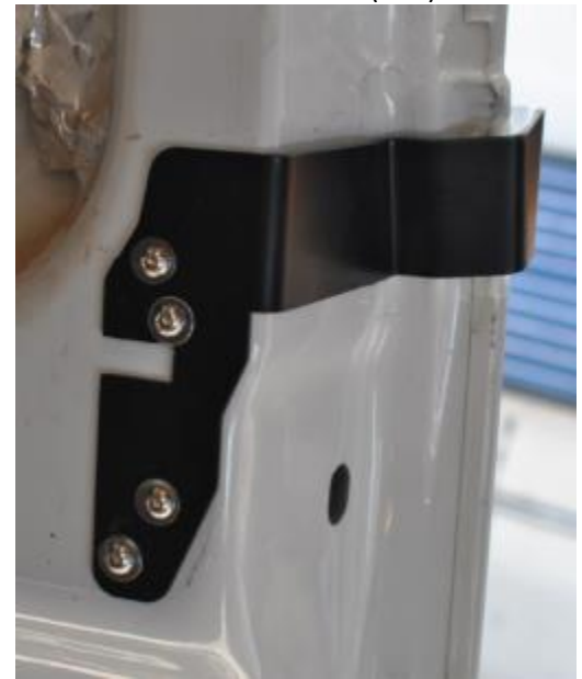
Figure 12: Installed Inside Upper Bracket without Factory Handle
