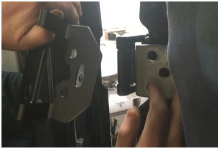
Figure 2: Upper Hinge Rotated Away from Door
