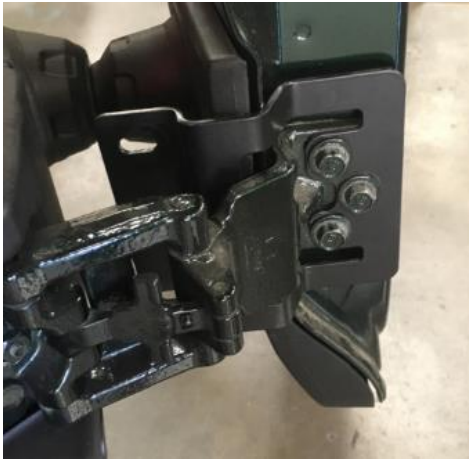
Figure 6: Inside View of Installed Lower Hinge Bracket
