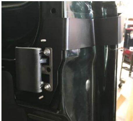
Figure 15: Upper Inner Passenger's Side Bracket Installed
