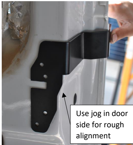
Figure 11: Dry Fit Bracket Up to Door
