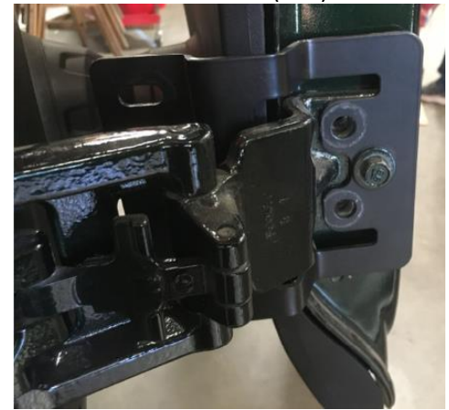
Figure 4: Hinge Placed Back into Position
