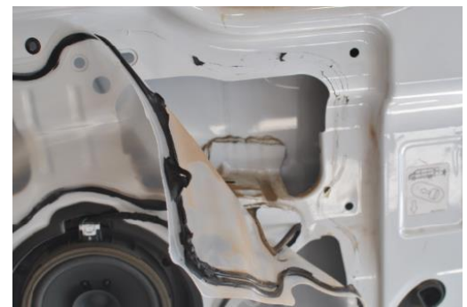
Figure 10: Inner Door Liner Peeled Back for Access
