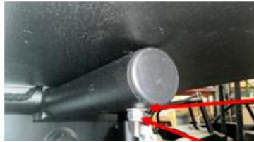
Figure 17: Mounting Hardware Under Box
