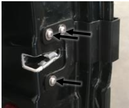
Figure 8: Installed Inner Passenger Door Bracket
