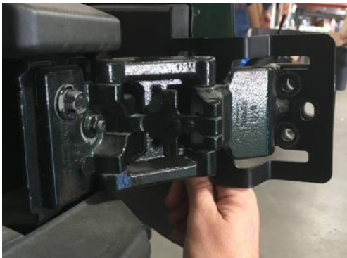
Figure 3: Bracket Installed Over Factory Hinge
