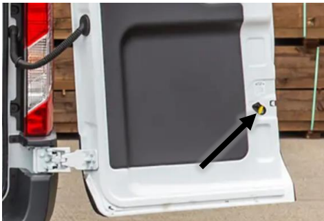
Figure 7: Inside Latch on Passenger Door
