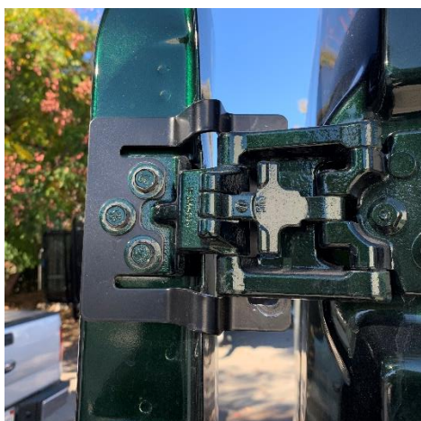
Figure 4: Inside View of Installed Upper Hinge Bracket
