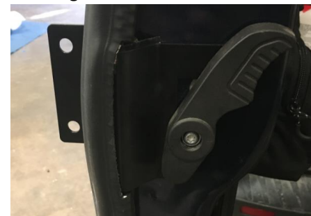
Figure 12: Installed Weather Stripping After Modification
