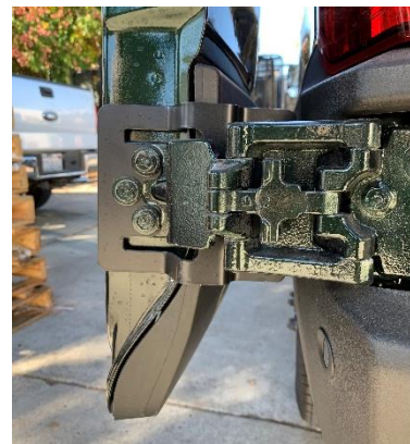
Figure 5: Inside View of Installed Lower Hinge Bracket
