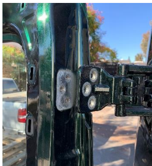
Figure 2: Upper Hinge Rotated Away from Door
