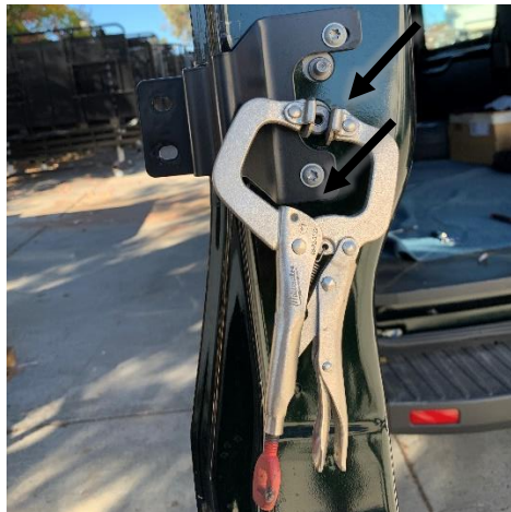
Figure 8 Inner Driver Door Bracket Installed
