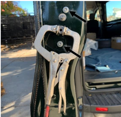
Figure 7: Removing Factory Torx Screws
