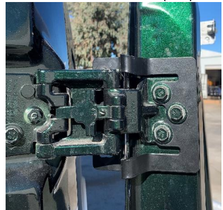
Figure 4: Inside View of Installed Upper Hinge Bracket
