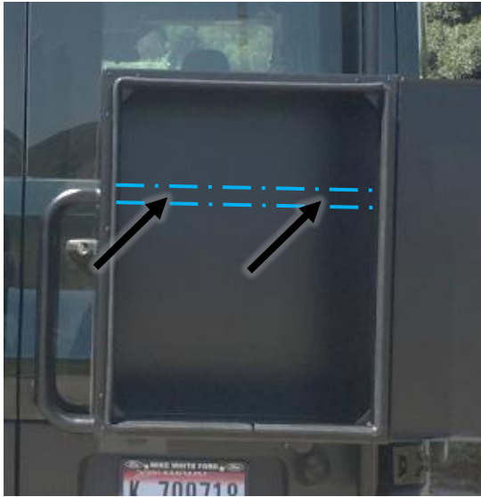
Figure 10: Mounting Box to Upper Cross Bar
