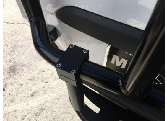
Figure 8: Bolt-On Supports Loosely Bolted to Lower Crossmember
