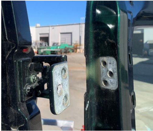
Figure 2: Upper Hinge Rotated Away from Door
