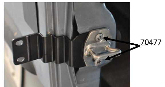
Figure 5: Driver's Inside Door Latch Bracket Installed
