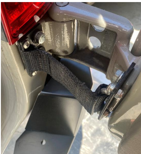
Figure 10: Limiting Strap Installed
