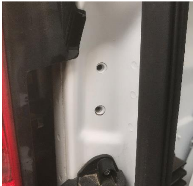
Figure 17: Factory Threaded Holes
