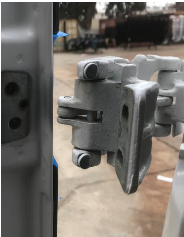
Figure 4: Upper Hinge Rotated Away from Door
