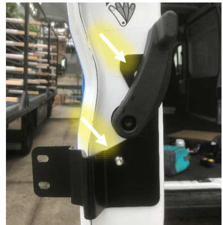
Figure 12: Inner Driver Door Bracket Installed
