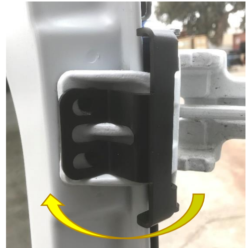
Figure 6: Bracket Installed Over Factory Hinge
