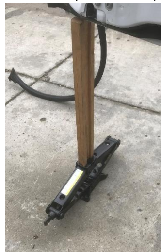
Figure 2: Support Door Prior to Installation
