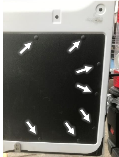
Figure 19: Remove Plastic Door Rivets
