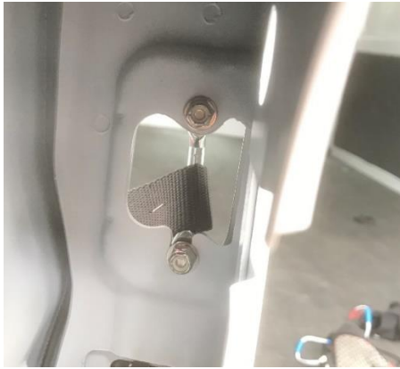
Figure 21: Backside View of Door Stop Mounting
