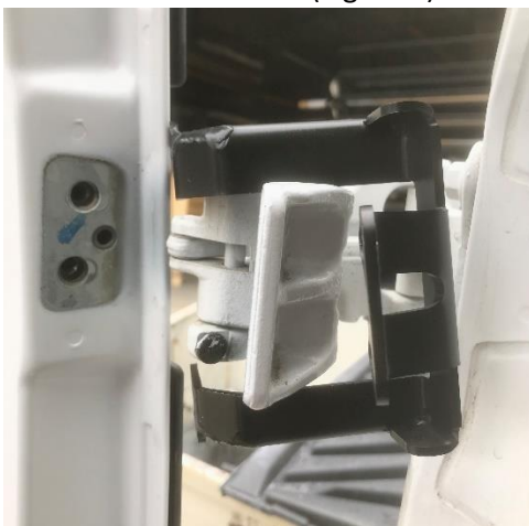
Figure 5: Bracket Installed Over Factory Hinge
