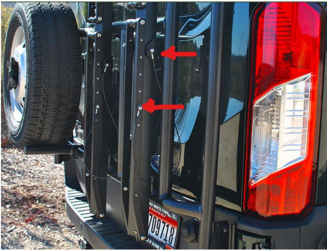
Figure 8: Steel Cable Location
