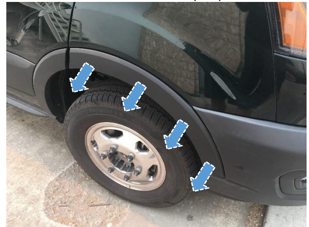
Figure 5: Fender Flare Removal
