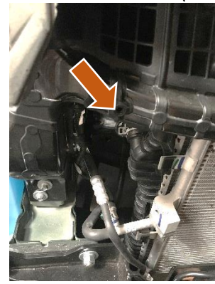
Figure 15: Upper Push Pin Location (Passenger Side Shown without Air Deflector)
