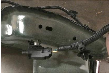
Figure 17: Temperature Sensor Removed
