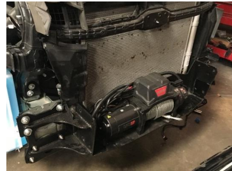
Figure 29: Winch Installed onto Winch Plate
