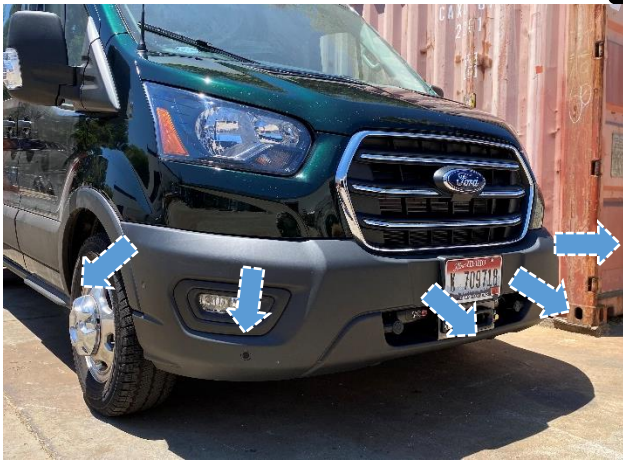
Figure 12: Factory Bumper Removal
