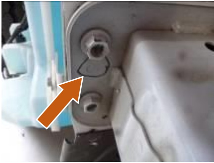
Figure 22: Example of Spot Weld (Shown from the Back)
