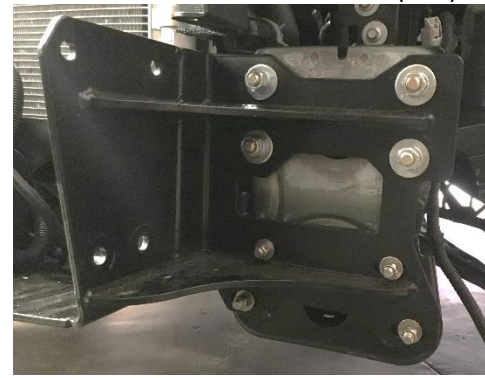
Figure 28: Winch Tray Installed onto Frame
