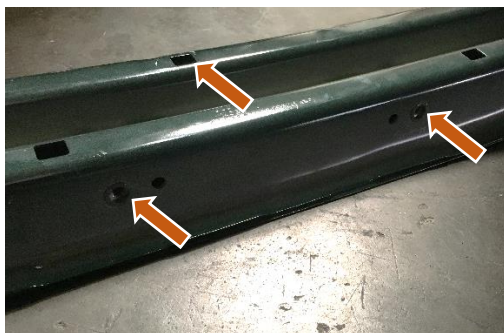
Figure 19: Front Radar and Bracket Uninstalled
