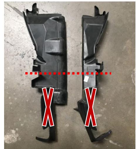
Figure 16: Radiator Air Deflector with Cut Line Shown
