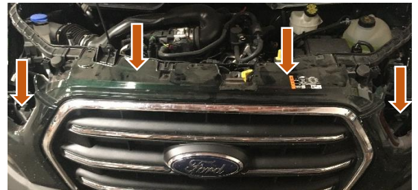
Figure 10: Locations of the Large Plastic Catches
