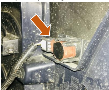
Figure 14: Parking Sensors from Backside of Bumper
