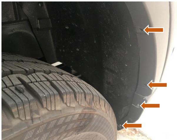
Figure 4: Torx Bolts Along Inner Wheel Well
