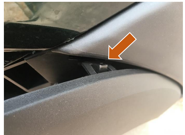
Figure 6: Fender Flare Plastic Clips Catches
