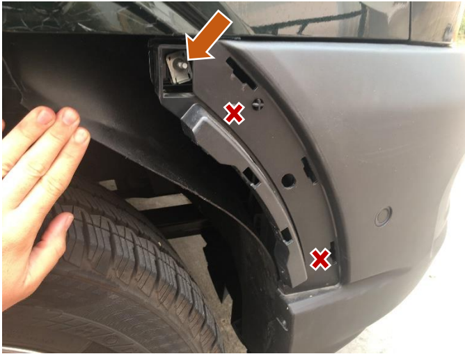
Figure 7: Bolt Accessed from Inside of the Wheel Well
