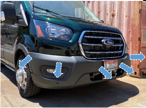
Figure 12: Factory Bumper Removal
