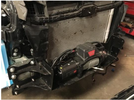
Figure 27: Winch Installed onto Winch Plate
