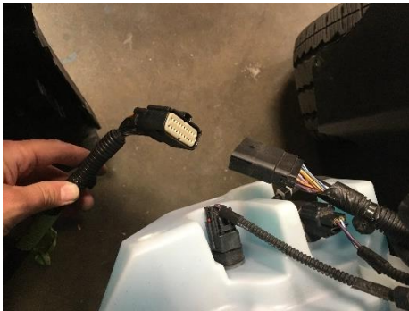
Figure 13: Sensor Being Disconnected
