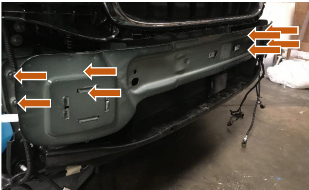
Figure 23: Lower Scuff Guard Removal
