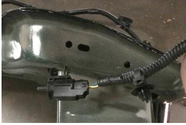
Figure 17: Temperature Sensor Removed
