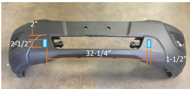
Figure 34: Tow Hook Cut Location
