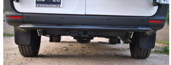
Figure 3: Hitch Clearance with Rear Nerf Step Installed
