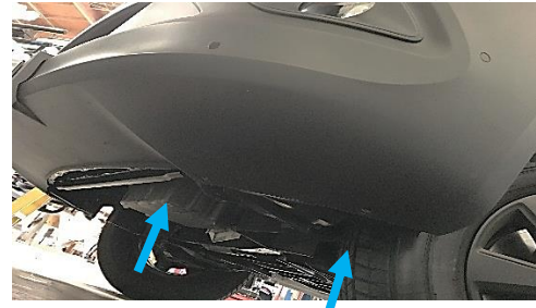
Figure 8: Plastic Rivets on Underside of Bumper
