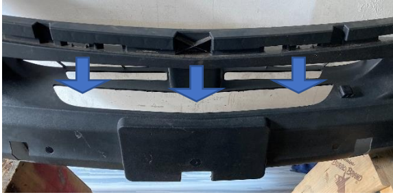
Figure 27: Factory Front Step Removal
