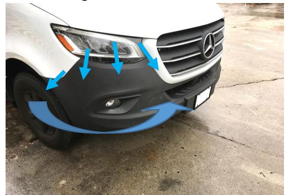
Figure 10: Removing Plastic Bumper
