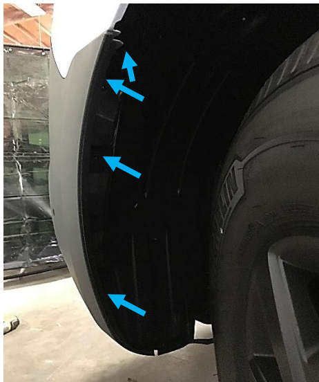
Figure 7: Plastic Rivets on the Inside of the Wheel Well
