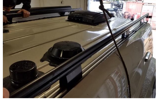
Figure 6. Remove drivers side rail once all bolts are removed.
