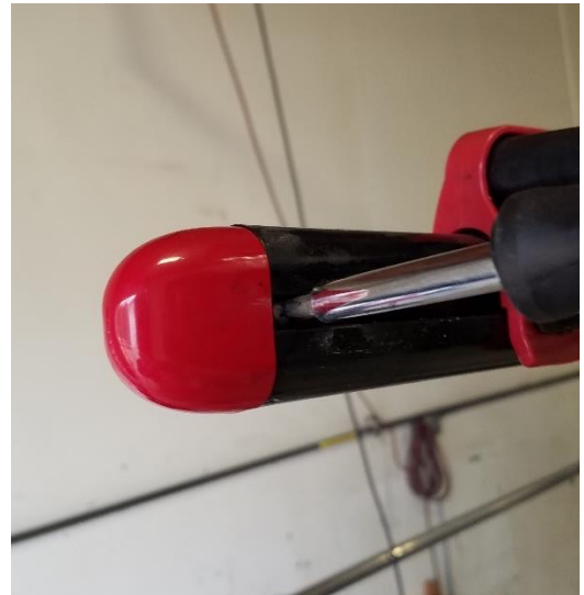
Figure 4. Removing end caps (red) from side rails.
