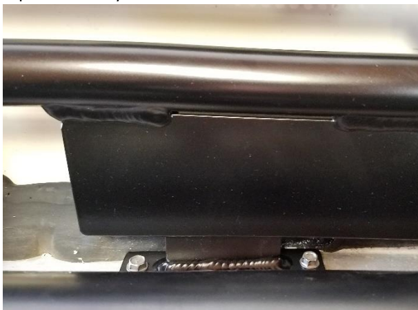
Figure 10. Installed awning channel bracket with roof rack placed on roof.
