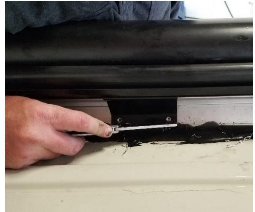
Figure 7. Drill out rivets and cut sealant around awning brackets to unmount one side of your roof rack.
