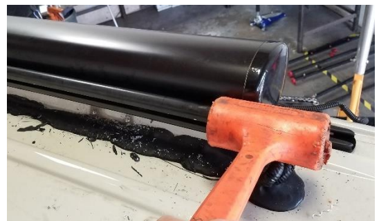
Figure 8. Remove passenger side rail.
