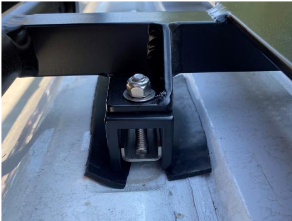
Figure 1: Promaster Roof Rack Mounting Installation
