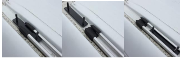
Figure 1: Threaded inserts installed onto tracks
